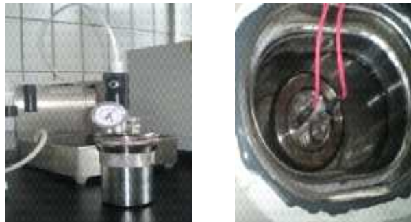
Fig. 2. Preparation of a „bomb” for examination ( a – filling the “bomb” with oxygen , b – placing “bomb” into calorimeter)
